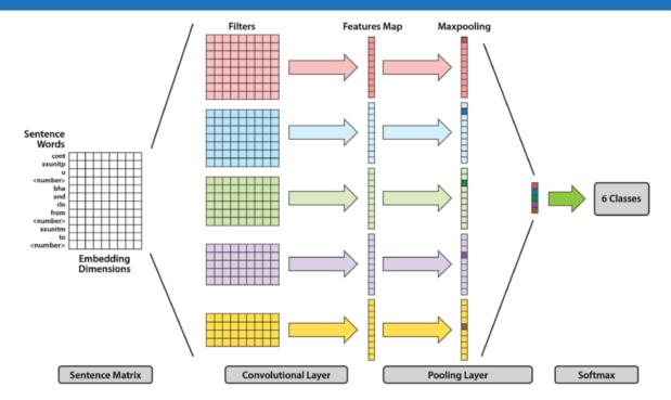
Given a sentence, a convolutional neural network uses convolutional layers to refine representations of input words, before combining them to render a classification.
