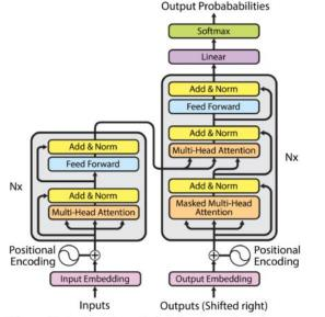
The encoder-decoder transformer used for translation. Encoder on the left, decoder on the right. Note that the decoder takes in its previously generated words during generation.
