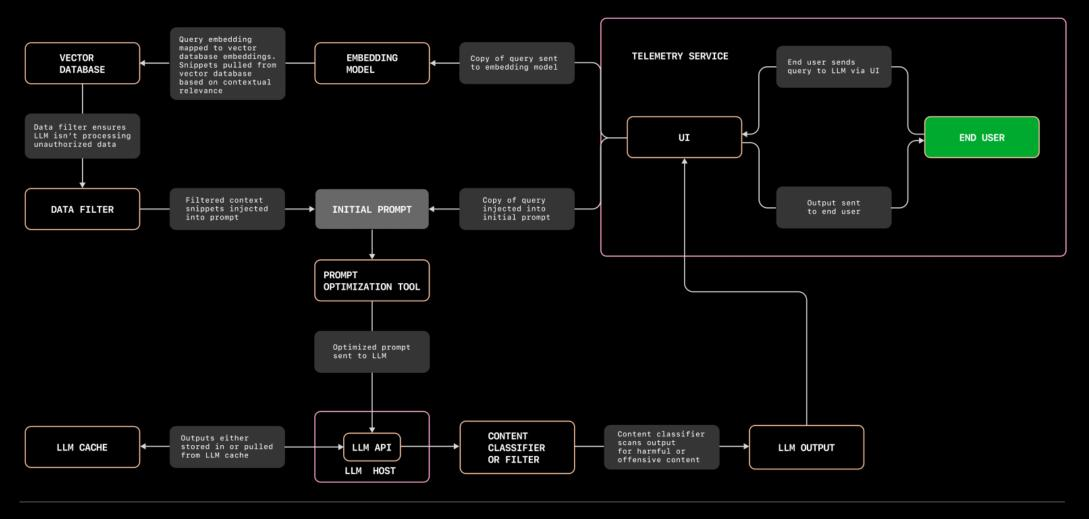
THIS DIAGRAM REPRESENTS THE ARCHITECTURE OF TODAY'S LLM APPLICATION. THE DIFFERENT COMPONENTS CAN BE ROUGHLY GROUPED INTO THREE CATEGORIES: USER INPUT, INPUT ENRICHMENT TOOLS AND PROMPT CONSTRUCTION, AND EFFICIENT AND RESPONSIBLE AI TOOLING.
